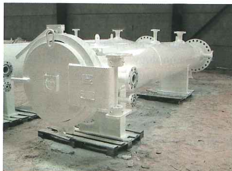
Pigs launching trap during the final finishing stage of construction at the plant in Puertollano (province of Ciudad Real) for the petrol-chemical complex in Ourhoud (Algeria). JGC Corporation (Japan) and INITEC (Spain) are developing the complex.
